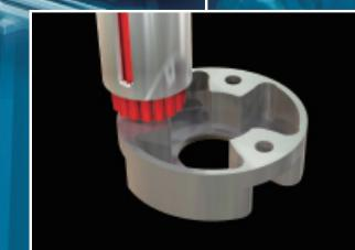
Part name **Housing** Tool used **XE BEC Brush™ Surface A11-CB40M**
