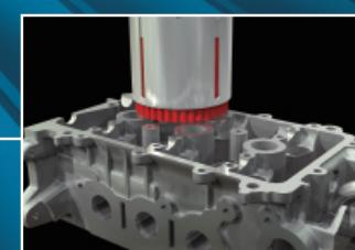
Part name **Cylinder head** Tool used **XE BEC Brush™ Surface A11-CB100M**
