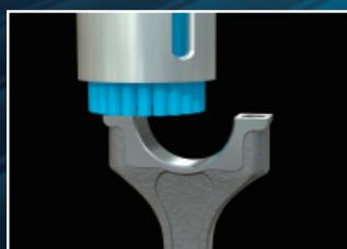
Part name **Connecting rod** Tool used **XE BEC Brush™ Surface A31-CB60M**
