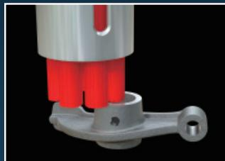
Part name **Rocker arm** Tool used **XE BEC Brush™ Surface A11-CB40M**
