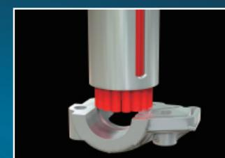
Part name **Cam cap** Tool used **XE BEC Brush™ Surface A11-CB40M**
